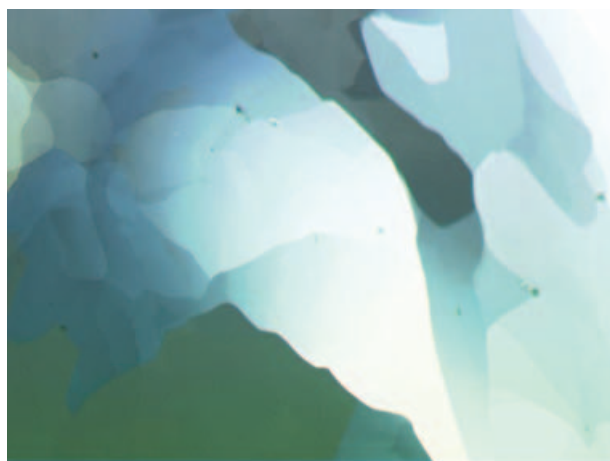
Figure 9. The platelet texture of the \text{SmB}_{\text{hex}} phase of 18a at 208°C.
